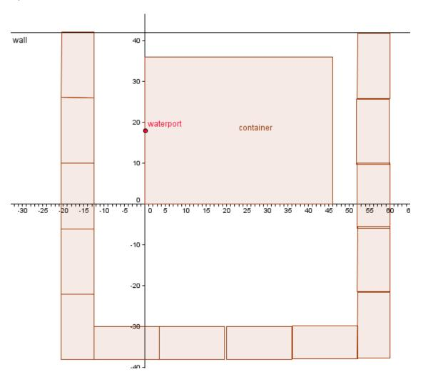
The cinder-block wall should be three blocks high and stacked directly on one another to avoid cutting a cinder-block. I didn't find a possible way to cross the blocks without needing to cut one.
