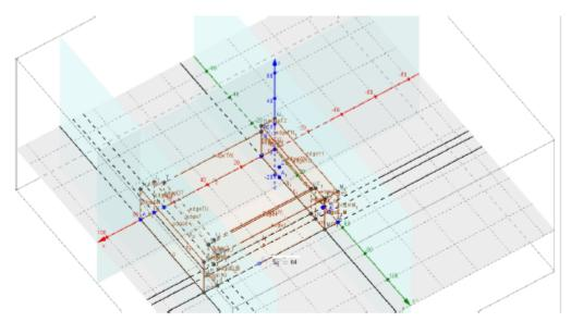
In order to accommodate the width of the air vent and provide the additional 8 inches needed beyond the physical unit, the width must be at least 44 inches. If we have internal lengths 58 and 44, to have a volume of 30 cubic feet (215 gallons), the height must be at least 21 inches.
